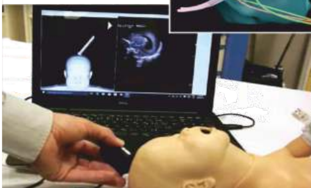
Head US simulator using VR and phantom technology
